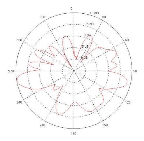
Vertical radiation pattern of BS 800, at 870MHz, measuring in a free space
