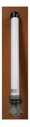
The wideband omnidirectional antenna requires no tuning. The antenna covers the whole UHF radiocommunication band. The antenna is designed for vertical polarization and is resistant to climatic conditions. The antenna is DC-grounded, there is an earthing clamp on the body of the antenna. In lower locations the antenna requires no additional lightning protection. Cast aluminum alloy base enables easy installation on vertical or horizontal elements of the mast.
