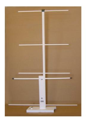
The antenna designed to base stations in mobile radiocommunication networks. The duraluminium welded construction is covered with powder varnish. The antenna is DC-grounded what ensures a resistance to all environmental conditions with a special consideration of highland installations, difficult-available high masts and unattended systems.
