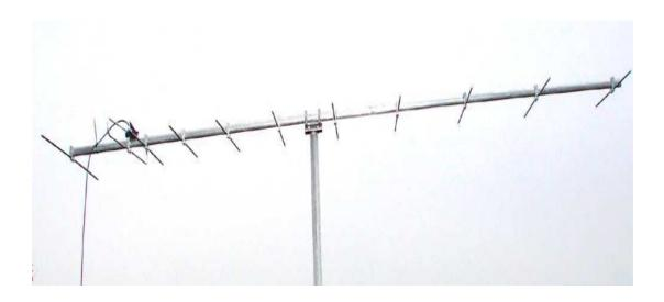
A typical 11-element Yagi antenna matching with a loop. A duraluminium construction may be fold out to transport. All screw connections are made of stainless steel, a PA7 alloy ensures required stiffness. A practical mounting enables install at vertical and horizontal polarization. Dimensions of antenna were optimized with a special consideration of wide bandwidth and keeping a high gain. The antenna may be produced for another frequency from the range  $140-460\,\mathrm{MHz}$ .
