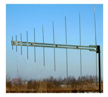
The wideband antenna designed to cooperate with radio direction-finders, without an additional tuner amplifier the antenna may cooperate with the VHF/UHF radio stations. The antenna mounting enables instal at typical vertical rotors.
